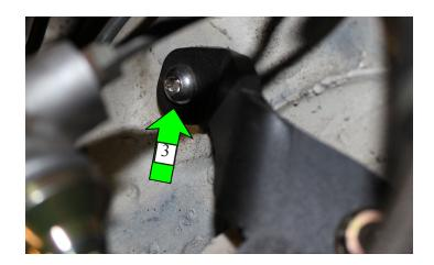
5. Position the gold foot on the end of the master cylinder. The end of it pivots to account for tolerances (both our tolerances and Mazda's), but try to make it as straight as possible. Tighten the front nut a bit to preload the brace, then tighten the rear one. Make sure the stud that the foot is on doesn't spin as you're tightening either nut, as that will change your preload.
