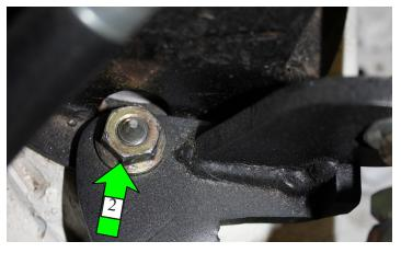
4. Loosely thread the bolt (with the small washer, the washer isn't shown in the picture) into the lower hole from step two (3), then reinstall the nut from step three (not shown here) and tighten it. Now, tighten the bolt from step two.
