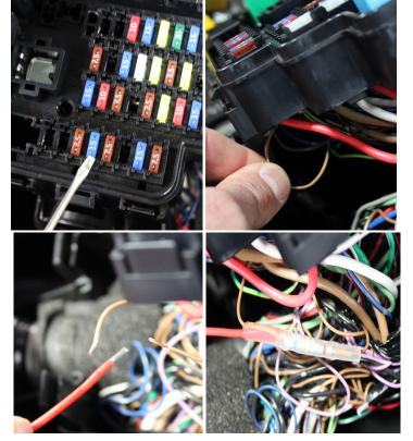
8. Locate the black wire under the fuse panel (3). It goes to the larger of the two connectors from step 1. If you have a ND2 with an automatic, you will not have this black wire and will need to use the black wire found below the ACC relay (4).
