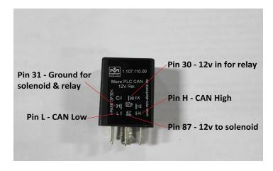
4. Here are the female spade connectors and MRS 9 pin connector block (07-44190). Pins 30, 31 & 87 will use the large spade. Pins L and H will use the small spade. Use the supplied wire, spades and block to build a connector for the relay. Pin 31 for ground will have two wires attached, one for relay ground, one for the solenoid ground.
