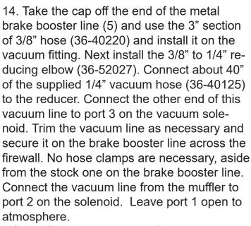
**NOTE:** If you are upgrading from the original control pack or adding this one to your existing Hush-O-Matic, remove the tee in the brake booster hose at the back of the intake manifold and put that plumbing back to stock. If your vacuum line from the muffler is too short to reach the solenoid you may be required to source a 3/16" (4mm) barb union and some additional vacuum hose to reach.
