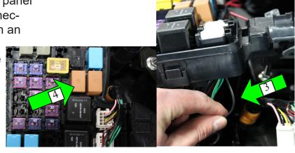
9. Tee the 8" ground wire from pin 31 into the black wire using another 3-way butt connector (36-80101). Use the same crimp/shrink method from step 7.
