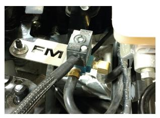
12. Take the two black wires from the vacuum solenoid and connect one wire to the 15" wire on pin 87 and other to the 15" wire on pin 31 on the relay using two red butt connectors (36-80100). It does not matter which is power or ground. Use the same method from step 7 to crimp and shrink the butt connectors.
