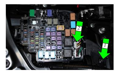
2. Use a small flat blade screwdriver to carefully pry the seven tabs while gently pulling up on the fuse panel to gain access to the wires underneath.
