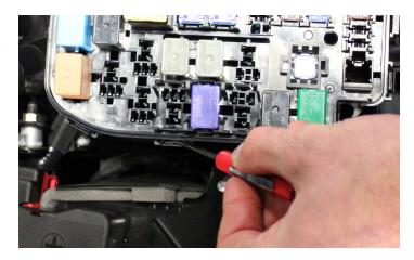
3. Here is the MRS PLC CAN relay (07-44110). The pins are labeled according to function. L and H refer to CAN Low and High.
