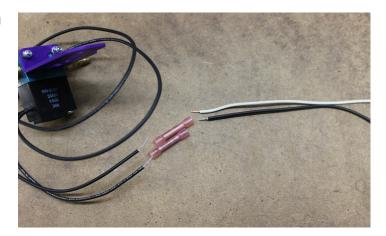
13. Locate the CAN communication wires under the engine bay fuse panel. They will be in the bundle of wires nearest the engine. They will be easy to find since they are the only wires twisted together. The black/blue wire is CAN high, the black/red wire is CAN low. Using two red butt connectors (36-80100) tee the black/blue wire to the 8" wire on pin H. Tee the black/red wire to the remaining 8" wire on pin L. Use the crimp/shrink method from step 7.
