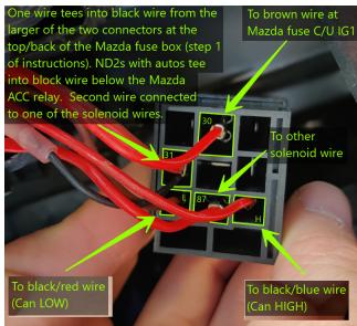
6. On the fuse panel locate the fuse labeled C/U IG1. Then locate the brown wire coming out from under it. Of the two wires connected to fuse C/U IG1 it is the wire nearest the firewall, farthest from the front of the car.
