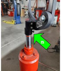
2. Install the tool onto the threaded post and tighten the retaining bolt with a 6mm Allen tool (5 - previous page). Do not overtighten as the bolt could begin to split through the Delrin, damaging the jack's threads.
